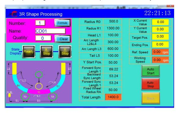
3R shape automatic processing steps: In "3R shape processing" interface, press the "PUMP" button, hydraulic station start, loosen the nut, the workpiece is placed into the machine, press "AUTO start" button, the middle roller moves to the rolling start point, then tighten the nut(no need very tight, suitable is ok), Again press to the
