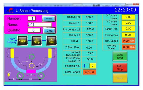
U shape automatic processing steps: In "U shape processing" interface, press the "PUMP" button, hydraulic station start, loosen the nut, the workpiece is placed into the machine, press "AUTO start" button, the middle roller moves to the rolling start point, then tighten the nut(no need very tight, suitable is ok), Again press to the "AUTO start" button, the machine automatically start bending processing. Repeat the
