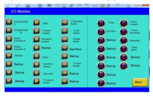
Through the "Diagnostic interface" interface can detect the input signal source (button, stop button, the grating ruler, rotary encoder) is normal, the output signal (solenoid valve, relay) is normal
