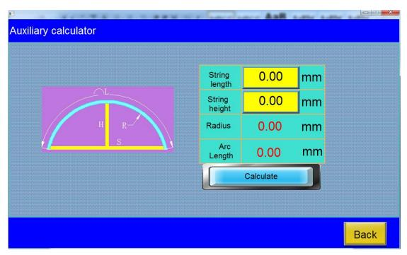
"Calculate" is for easy radius calculation in actual use, the parameters of arc is encountered, through calculation, provide the basis for practical use;
